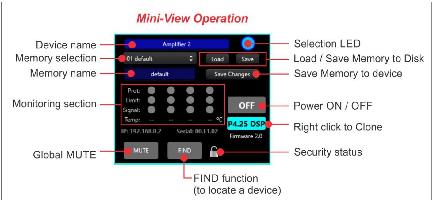
The active amplifier has a blinking blue LED on the top right corner of the mini-view (The front panel of the active amplifier has his POWER button blinking at same speed than the software). To select an amplifier, left click on the Selection LED. To edit the parameters of the active device, click on the Top bar control buttons (Input, Output, Mixer, Sys). Each mini-view can be moved on the desktop simply by click & hold operation.
