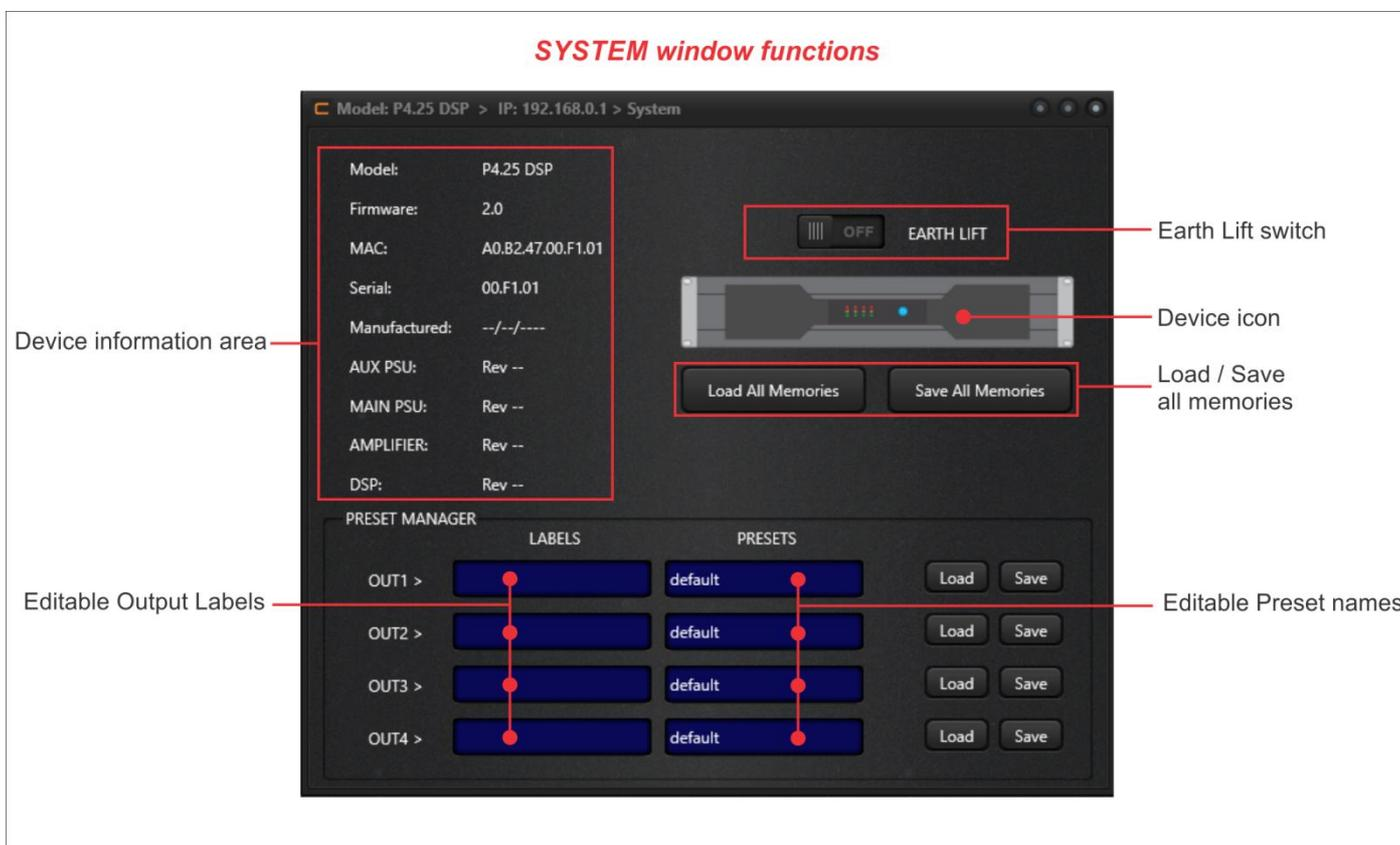
**Remark:** like MUTE, EARTH LIFT state is not saved into memory. When the amplifier starts, it's always OFF.
